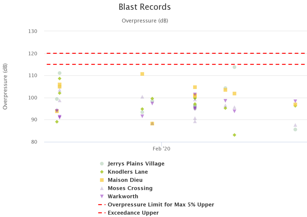
Figure 9: Overpressure Blast Monitoring Results – February 2020
