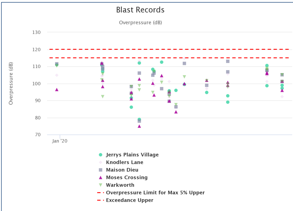
Figure 8: Overpressure Blast Monitoring Results – January 2020
